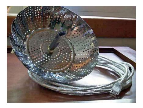
The garden shed is on the far side of the house from the wifi server in the house, so the signal is quite poor, but by sliding the antenna back and forwards on the USB wifi adapter, I could significantly increase the signal, and get good reception. I mounted the whole thing on plywood stand and took it to the boat.
