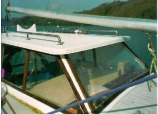
On deck we have been able to improve the appearance of the doghouse by taking the roof outboard by five inches and aft by three feet. A 15 stone crewman is able to walk on the rooftop, an opening hatch also allows the helmsman to sit on the roof and steer with his feet! There is also ample space here for life-raft stowage and solar panels. The plan now is to fit roll up awnings along the under side edges of this deck so that the cockpit can be completely enclosed.
