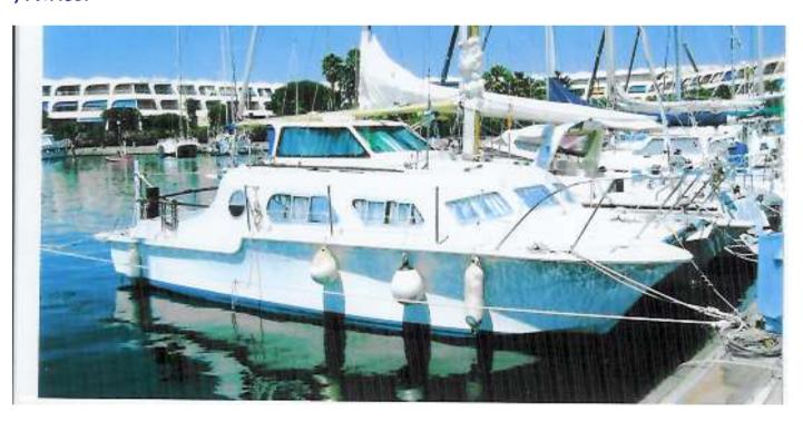
HULL Hull strengthened for cruising with 3 layers glass fibre (external) in Isopthalic resin and encased in epoxy (Professionally completed 1996)
